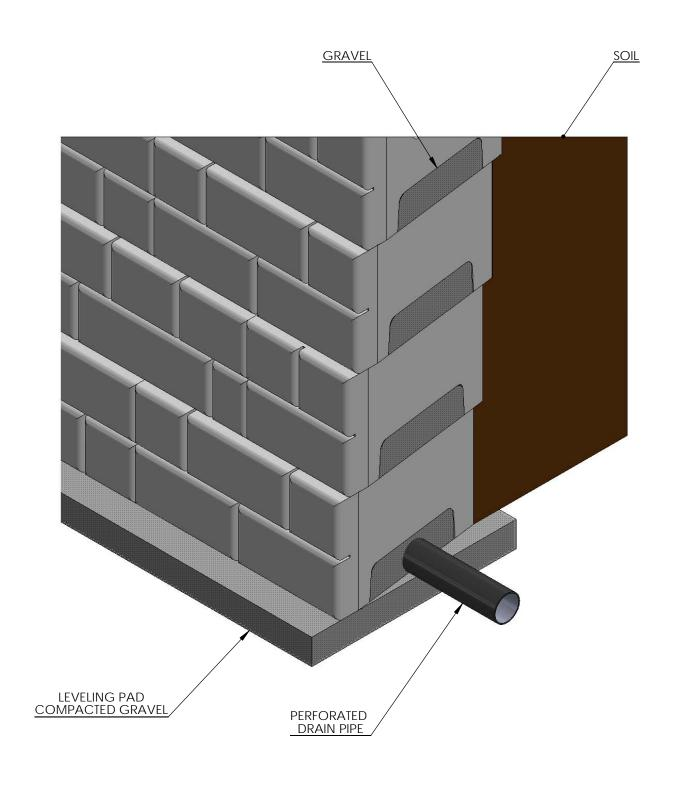
DRAIN PIPE IS PLACED INSIDE GAP AT THE BOTTOM OF THE BLOCK AND ON TOP OF THE LEVLING PAD THEN COVERED WITH GRAVEL.
